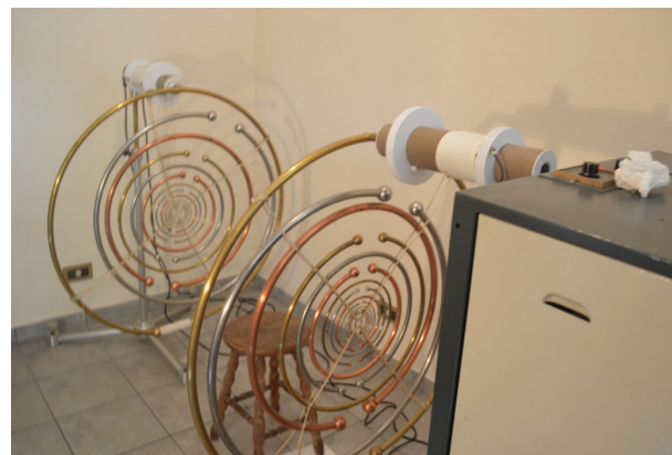
Figure 132.1 Lakhovsky MWO built in Brazil. We can see a coil adjustable in each antenna. The sparks in the antennas measure 2.5 to 3 cm.
