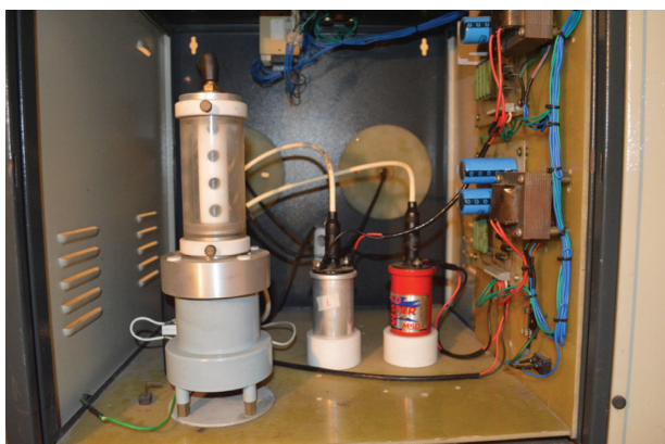
Figure 132.2 Inside view of MWO built in Brazil. The four sparklers are made of titanium.
